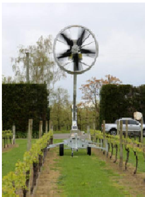
A towable wind machine that frost protects 4A
